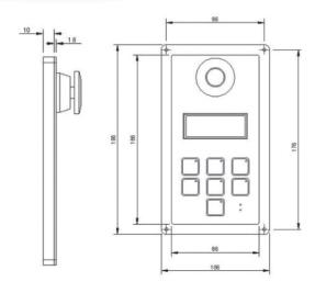
Control Panel is mounted on 10mm thick white acrylic frame, with 1.6mm MS bracket powdercoated white.
