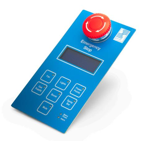
A fume cupboard with an **EcoAir® III Controller** is a variable air volume (VAV) system. The Controller monitors the sash position and continually adjusts the fan speed to maintain a constant face velocity as the sash height changes.2 The EcoAir® III Controller thereby saves energy and improves HVAC efficiency by exhausting less conditioned air from the laboratory.
